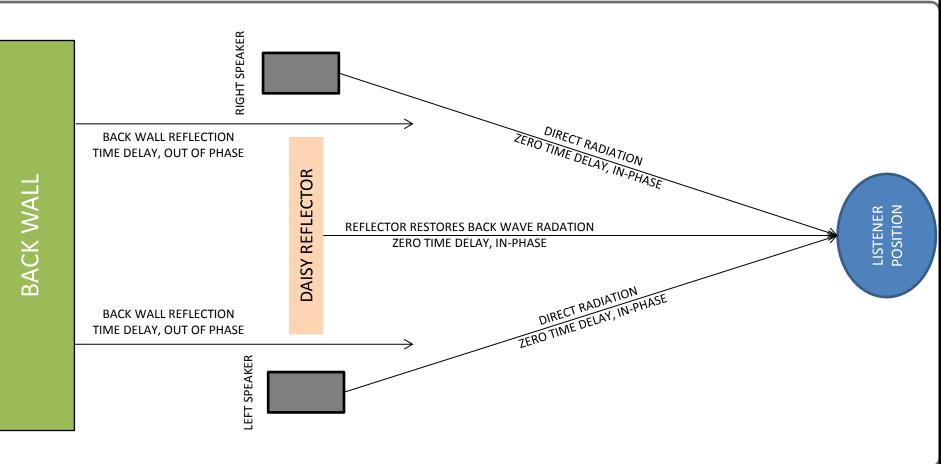
The Daisy Reflector is a substitute to the back wall, within the window that generates the first frontal arrival waves. Because of position and shape alteration it produces a 3 axis time alignment of the reflection. The result is phase and time coherence of the total frontal wave.
